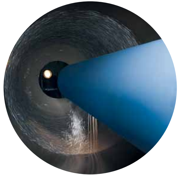
Centrifugal casting process patented by HOBAS
