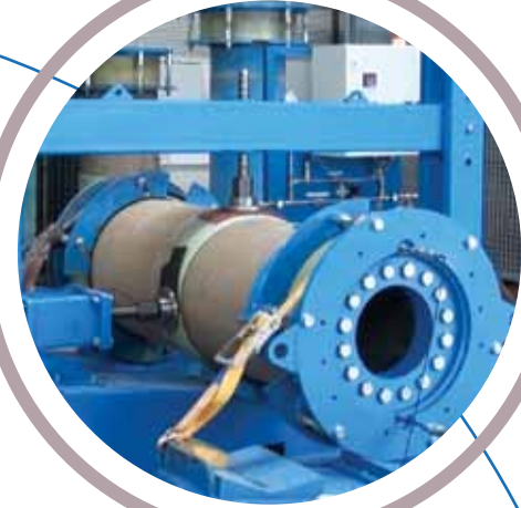
Testing the angular deflection in couplings
